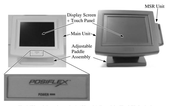
The MSR unit is option to both 12" and 15" models. The LED in the logo area serves for multiple purposes through giving different indication of steady/flashing green/orange light. Please refer to the paragraph discussing the LED indication in the chapter of "USING THE TOUCH POS" of this manual.
